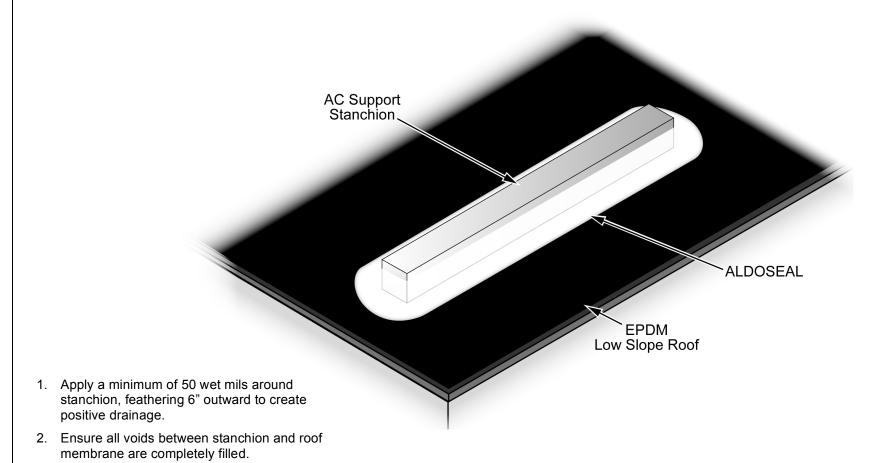
Note: Support stand must have remaining service. If deteriorated, it must be replaced and membrane repaired prior to ALDOSEAL application.
