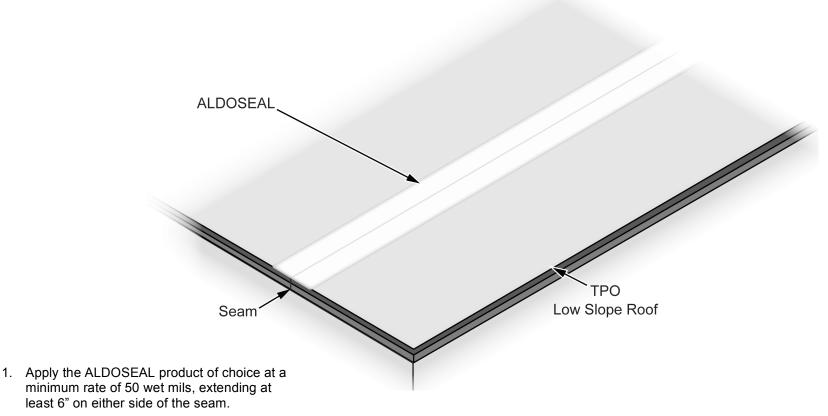
2. Ensure that product fills any seam void or opening completely.
